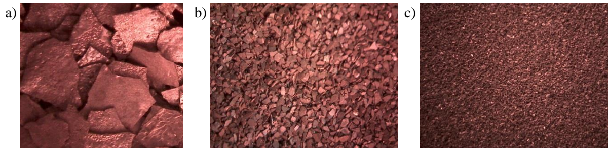
Fig. 4. Appearance of scale samples after 1 hour of grinding (x 50): a – scale with a fraction of 1-1.2 mm; b – scale with a fraction of 0.4-0.315 mm; c – scale with a fraction of 0.2-0.16 mm
