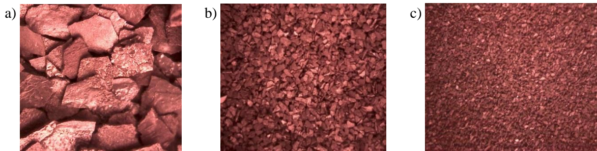
Fig. 5. Appearance of scale samples after 2 hours of grinding (x 50): a – scale with a fraction of 1-1.2 mm; b – scale with a fraction of 0.4-0.315 mm; c – scale with a fraction of 0.2-0.16 mm
