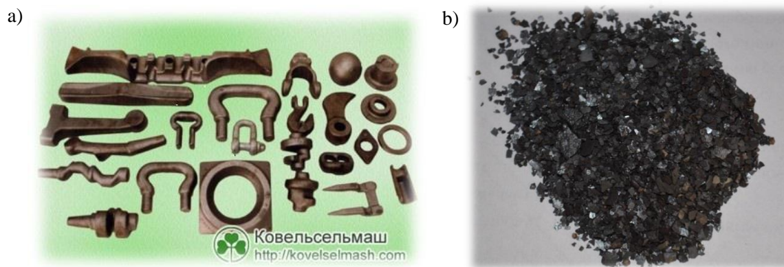
Fig. 1. Parts produced by hot plastic deformation (a); scale particles (b)
